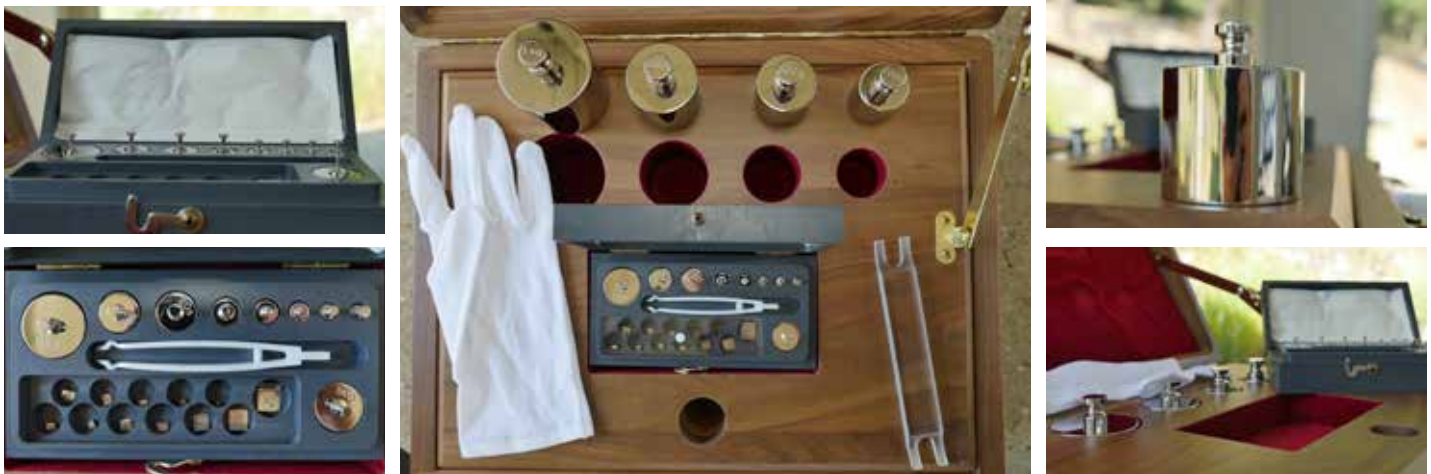
Class II test kit, 1mg to 1 kg
